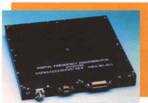
Fig. 1. A miniature DFD for airborne applications.
